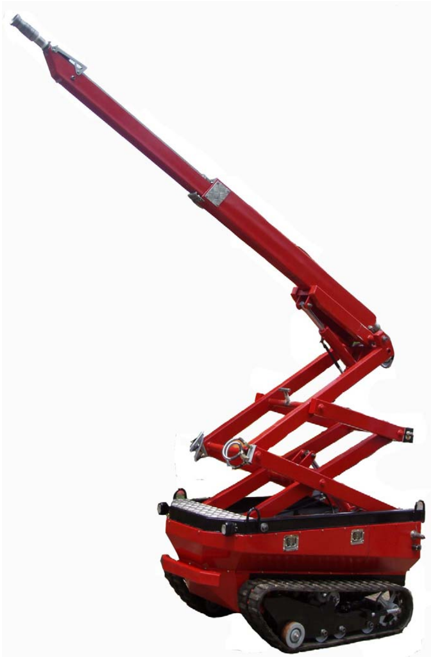
Figure 6 MyBOT 2000 with full extension of elevated fire hose
